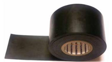
Polygomma<sup>™</sup> EPDM Strips can be used to seal the joint between façade/window and the adjacent structure. It not only waterproofs the critical joints, but also makes it air-tight, and protects against moisture. They are also used as a Damp Proof Course (DPC) and for expansion joints.
